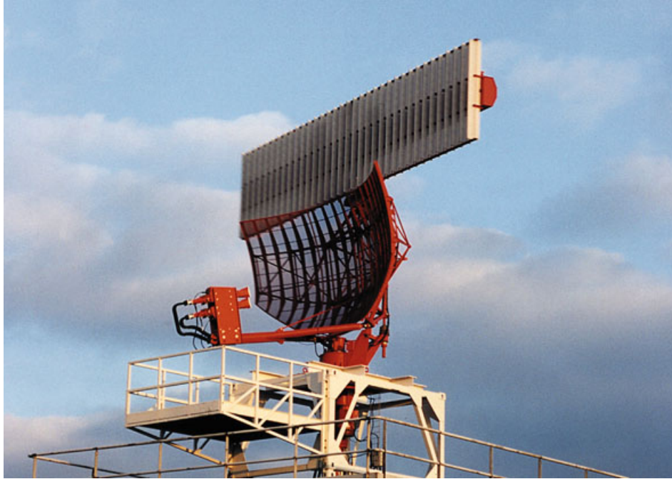
Figure 4: Primary and secondary co-mounted radar antennas
